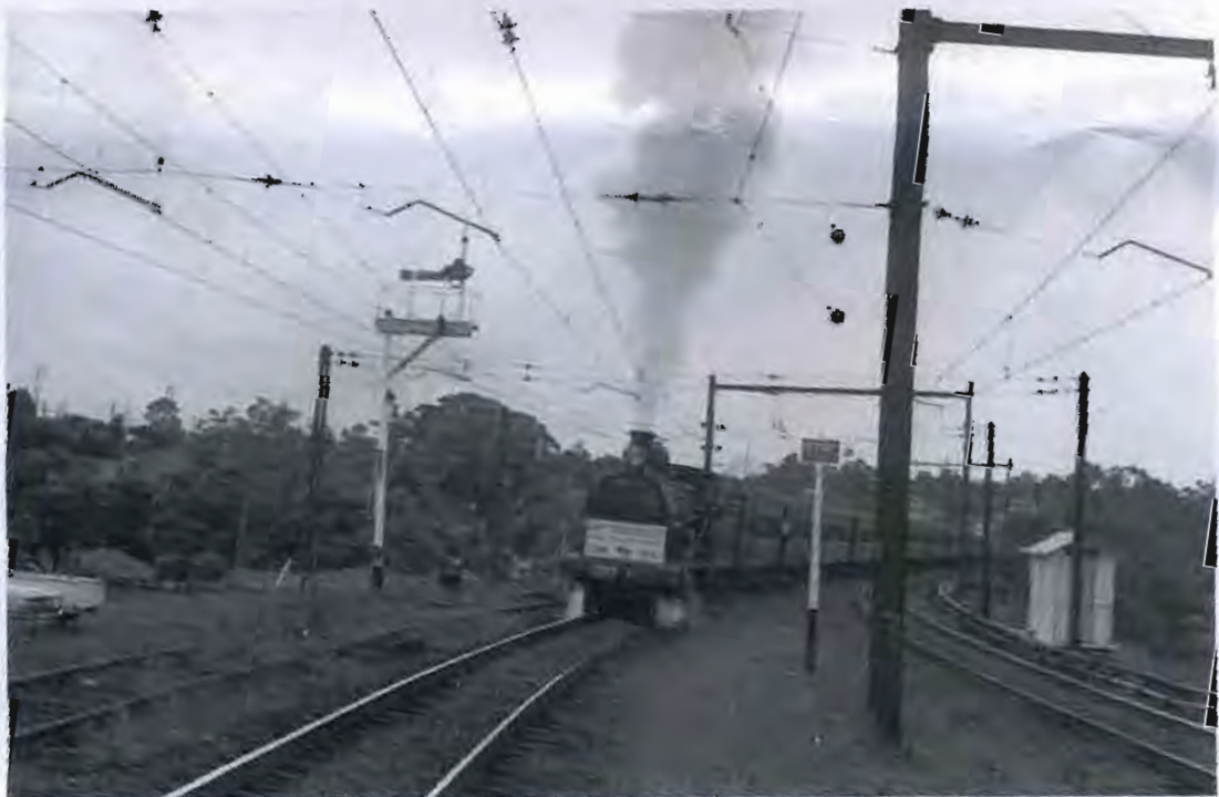
Looking south from platform. The Engine Siding is on the left. The locomotive has propelled its train out of the Engine Siding and is now heading in the Up direction on the Down line. Note that the Engine Siding is electrified. Note the banner signal on the Engine Siding. The upper quadrant semaphore signal serves the Down Main. Oatley 29 February 1976 Alex Grunbach RRC 209523
